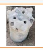
When drilling in non-abrasive materials, where carbide wear is minimal, extended drilling intervals are possible. This allows for prolonged chip removal around the bits and will wear away the bit body to a greater extent than the buttons. Similar wear occurs in fractured and loose materials where excessive agitation and grinding of the materials is required for hole cleaning and to keep the hole open during retraction. To prevent tearing out buttons and
